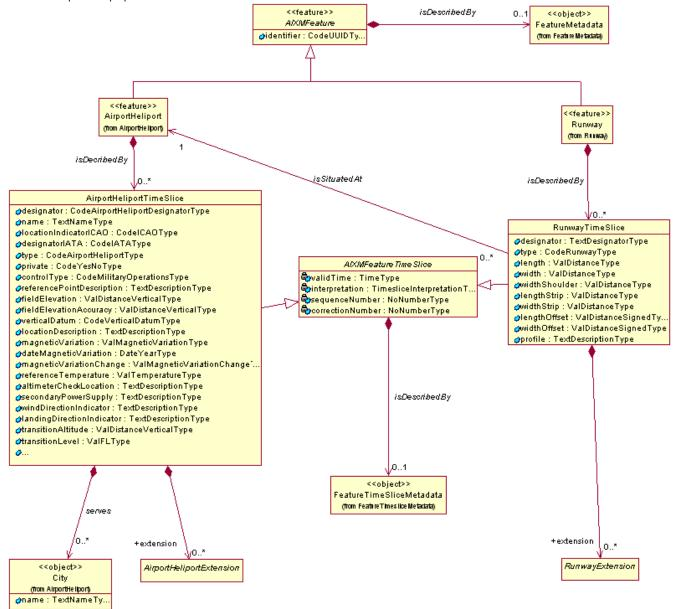
The diagram above is quite complex. If applied to the whole set of AIXM classes, it might undermine the readability of the UML diagrams. Therefore, the Design Team has decided to provide a simplified UML model, without visible inheritance of all features from the abstract AIXMFeature and without visible SomeFeatureTimeSlice classes.
